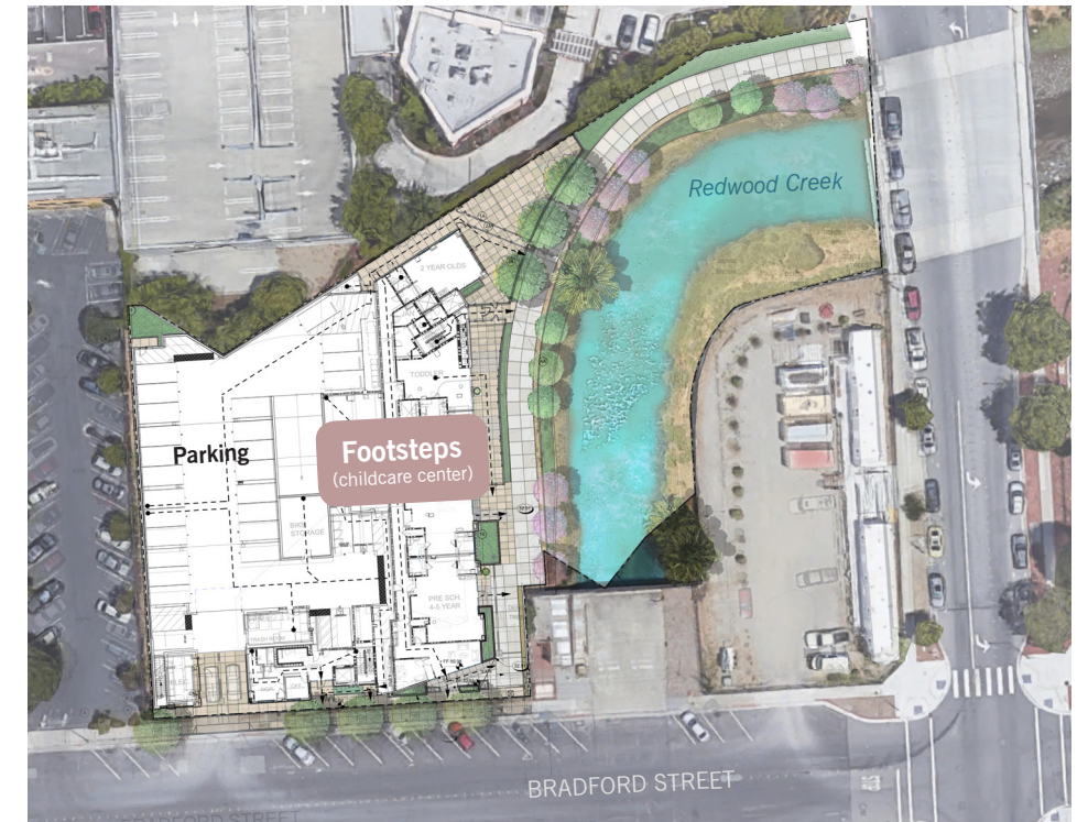
A second level of parking was added to the building, as a result of unsuitable soil conditions for underground parking. The vertically mixed-use building places senior living over Footsteps, a childcare center, combining uses that promote intergenerational programs for mutual benefit.
